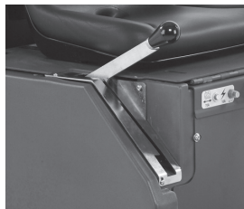
Mechanical deck lift lever.
