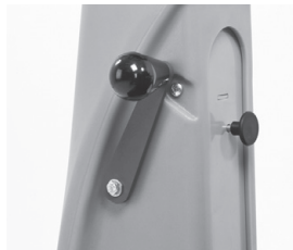
Mechanical squeegee lift lever located on steering column.
